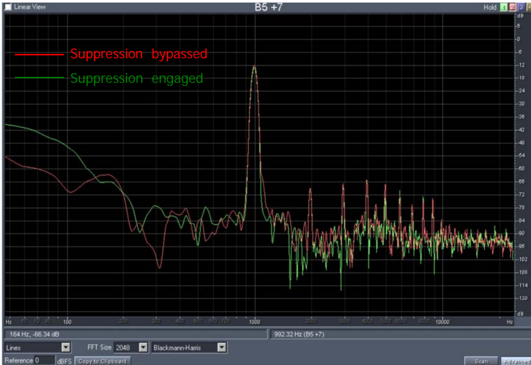
Figure 8: FFT plot of MIO System, HATS left, ping tone plus decay envelope
