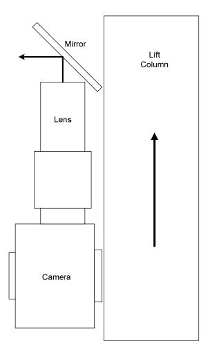
The camera lift column can be raised and lowered depending on whether the student would normally be sitting or standing to play a particular instrument. Similarly the workstation used by the student to view the panoramic video will be able to be raised and lowered to the correct position.
