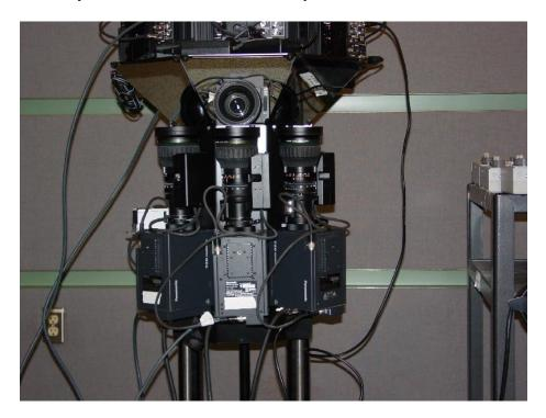
The lift column is mounted on a base with casters for easy movement to different positions without the need to re-align the cameras.
