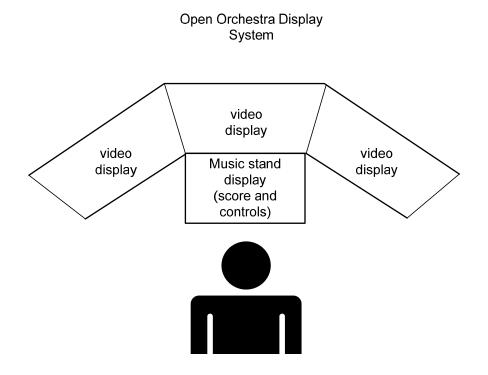
The problem with acquiring three simultaneous video streams for display in this manner is that all three cameras must be co-located where the student would be to give the correct visual perspective on each screen. This is a major challenge given the size of the high definition broadcast cameras and their lenses and the need to see objects that are very close to the student.
