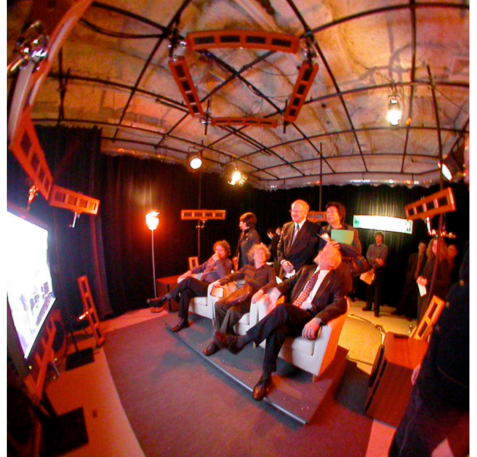
Figure 4. Three chairs on a motion platform with a view of the plasma screen and multichannel loudspeaker system for experiments in interactive telepresence with immersive reproduction of sound and vibration.
