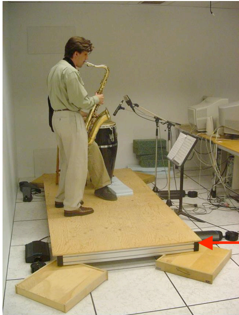
Figure 5. Vibrational signal transmission using motion platforms. The arrows point to the platforms. The audience can feel the vibration generated by musicians in the studio.
